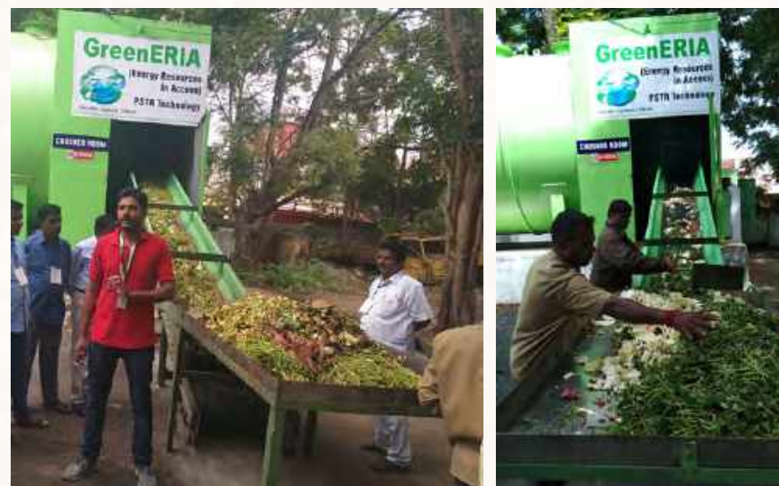
Organic waste passed to the shredded through the conveyor belt
