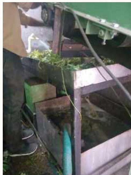
Organic waste shredded to form slurry to feed into the Digester
