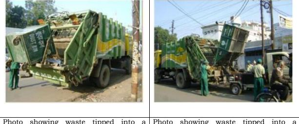
Photo showing waste tipped into a<br/>compactor truck from a collection bin in<br/>KanpurPhoto showing waste tipped into a<br/>compactor truck from an auto tipper in<br/>Kanpur
