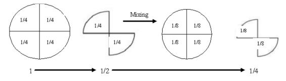
Figure 3.2: Sampling Procedure through Quartering Method
